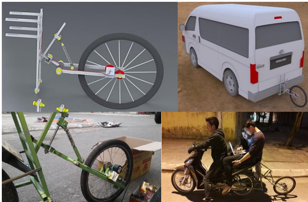
Figure 10.1: Images of the product of student research project "Study on design an equipment to measure the velocity of automobile and motobike" is used to measure the speed of cars and motorcycles in the course "Automobile testing"
